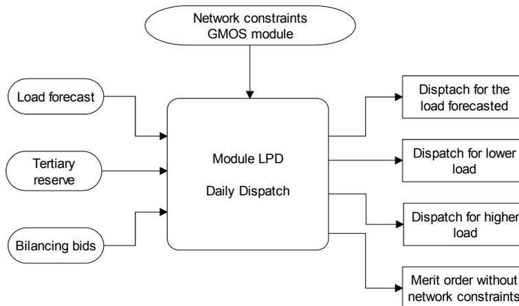
Fig. 12 Input and output module for LPD program
