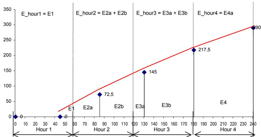
Fig. 10 Allocation of start-up characteristic in one hour intervals.
