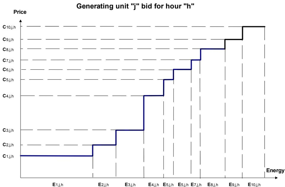
Fig. 6 Graphical representation of a balancing bid
