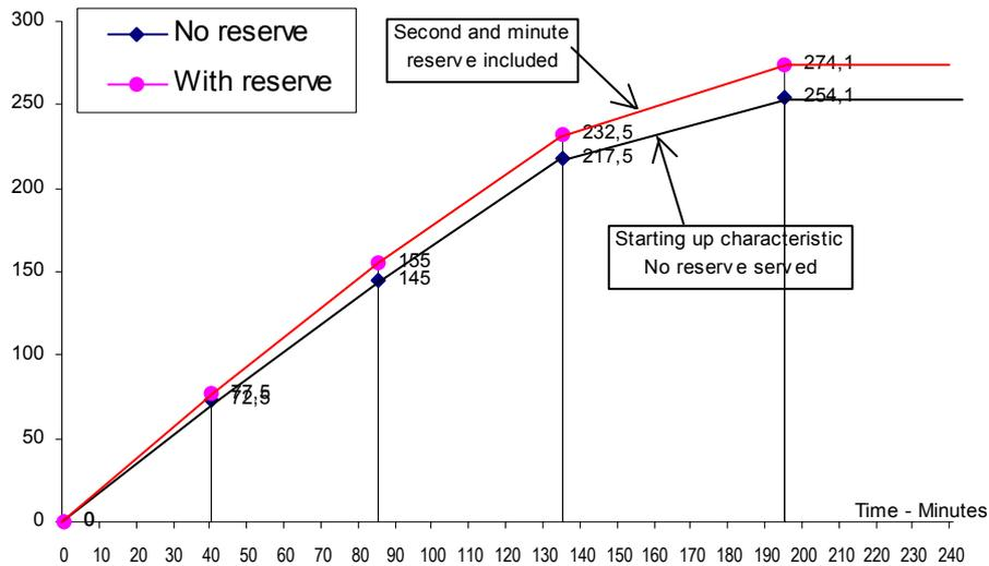
Fig. 8 Start-up characteristics of a generating units.
